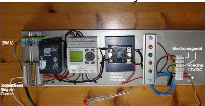
Below the bottom plate we have a floor-pit with a 230 VAC supply and the signal wires coming from the topmount. Connections are visible on the left side. On the right side a 12 Volts DC supply (unit not on the photo) enters for the electromagnet.
