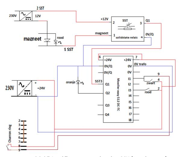
2.3.4.5.6 and 7 are connected to the +24V from the transformer. PLC is Moeller easy 512 DC-TC
